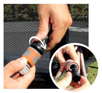
At the base of the net pole, connect the MeteorShower<sup>™</sup> tube and garden hose together using the hose adapter supplied in the MeteorShower<sup>™</sup> kit.
