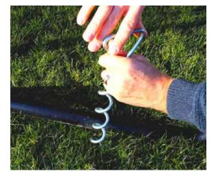
Set the anchor adjacent to a trampoline foot, then press down and turn clockwise to puncture the ground. Continue turning until no coils remain visible. STEP 2
